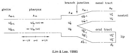
• Transfer function is adequately represented by a Pole-Zero model
